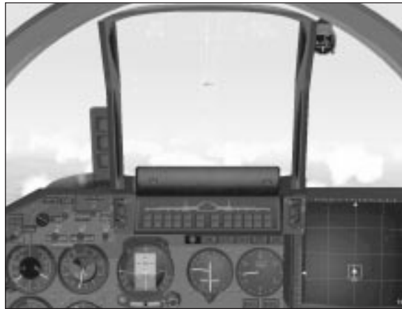
6-3: The Autotrack HUD Symbology (Range > 1400 meters)
