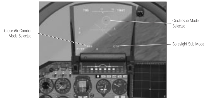
4-10b: The Radar Bore Site Mode Close Air Combat Symbology
