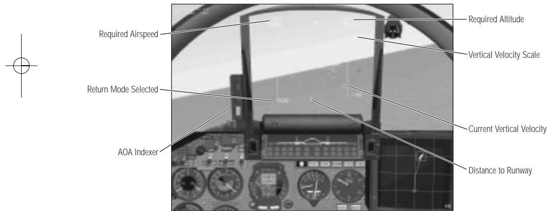
4-6: The ПОО -(LNDG) Landing Submode with ILS
