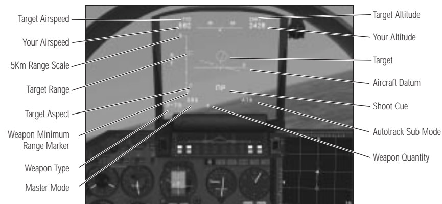
4-15: Autotrack Symbology with Radar Lock
