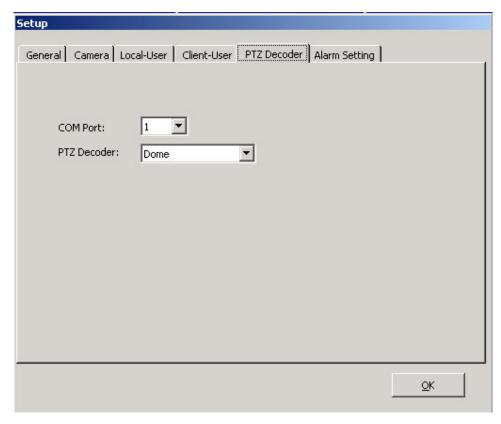
COM Port: Choose the communication port that your RS232 to RS485 adapter used, RS485 adapter connects to your PTZ decoder.
